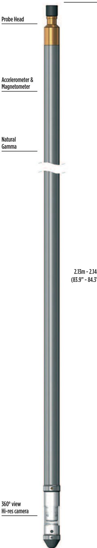
The High Resolution Optical Televiewer (Hi-OPTV) provides a continuous very high resolution oriented image of the borehole walls using a conventional light source.
