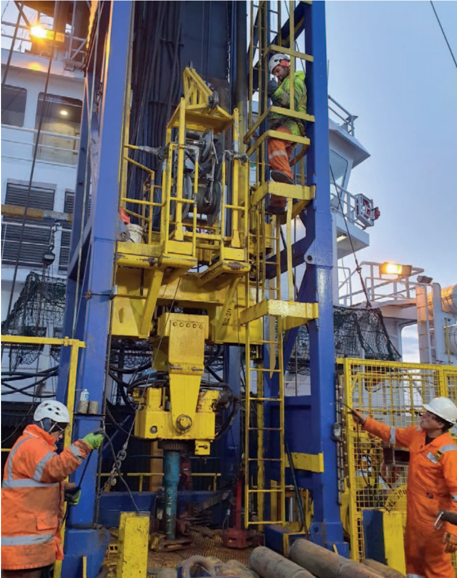
2,000m Marine Winch secured in a custom frame on the rooster box.
