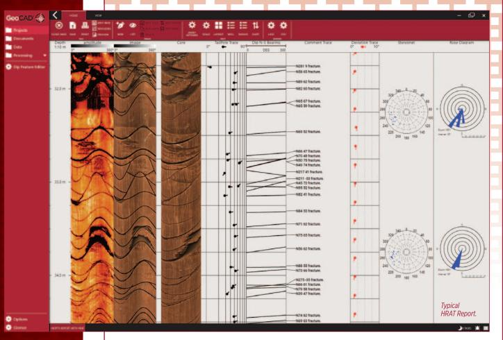
**GeoCAD®** is a windows-based package for processing, interpreting, and displaying acoustic and optical televiewer image logs. Standard log presentations include tadpole and stick plots, stereographic projections of poles to planes and azimuth frequency diagrams. The synthetic core display allows the convenient comparison of log and field data for the orientation of fractured or incomplete core sections.
