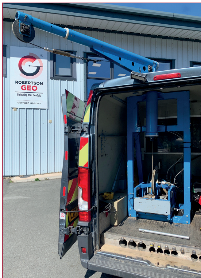
Figure 4: Van and Boom Arrangement.
