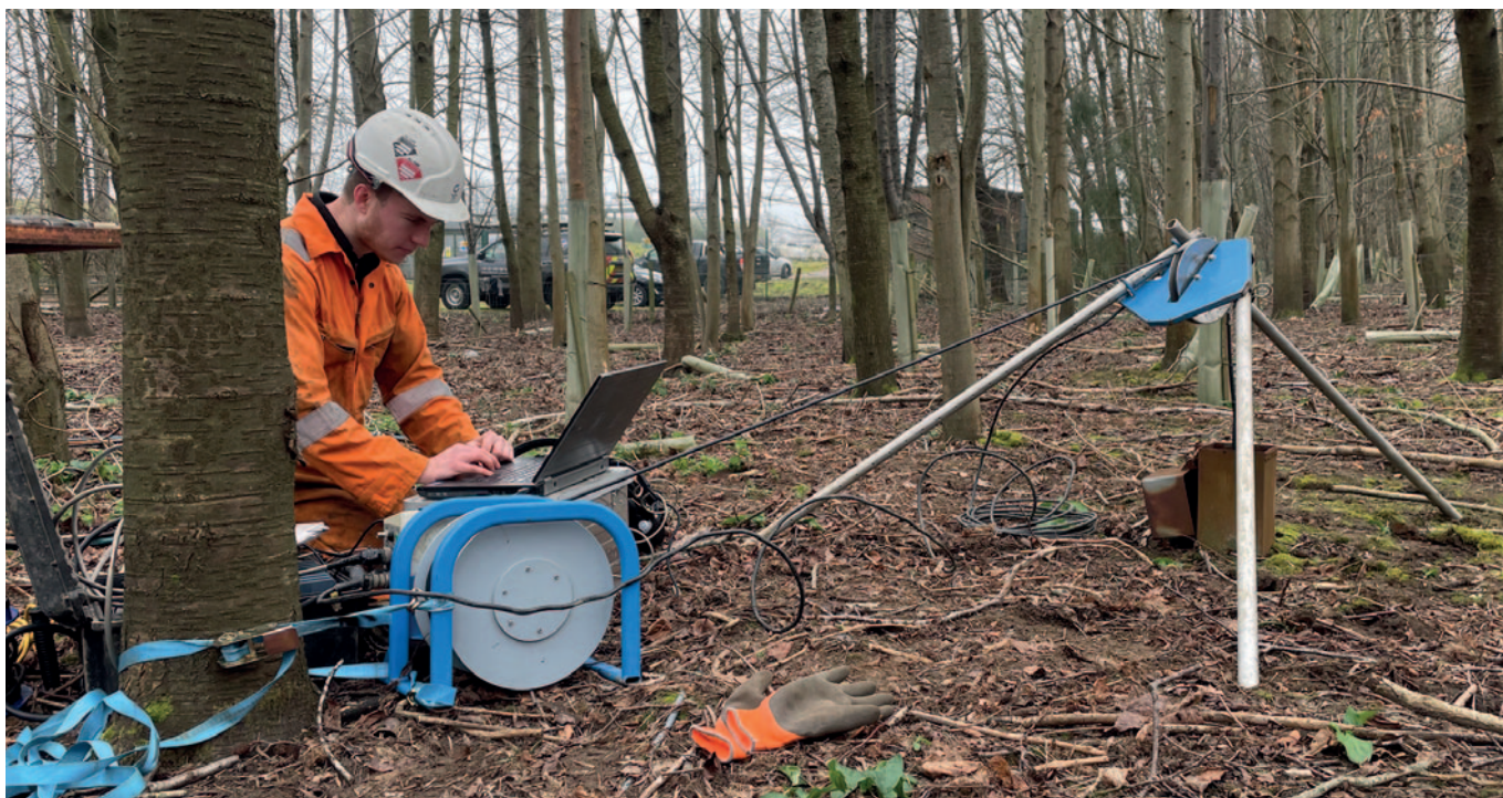
Above: Logging engineers need to be resourceful – here using a tree to support the winch during portable operations.
