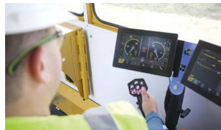
A drill outfitted with AutoTension allows HDDs on both sides of the bore to work together
