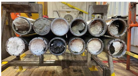
Samples collected by Benthic using thin kerf rotary corer Photo: Leonel Mello
