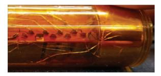
The probe does not require centralization, however, in inclined holes there is a risk of running the probe in a layer of collected sediments. Some form of stand-off might prove to be helpful in these conditions.
