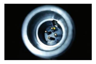
The area can be cleaned out with distilled water and then isopropyl alcohol if necessary, but should be allowed to thoroughly dry out before use (At least five hours open to the air).
