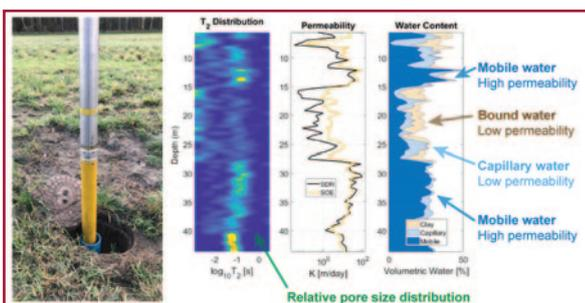
Vista Clara's advanced Javelin family of borehole NMR magnetic resonance logging tools provide direct, low-cost, high-resolution measurements of hydrogeological properties including: Volumetric water content; Pore size distribution; Bound and mobile porosity; Hydraulic conductivity and Transmissivity.
