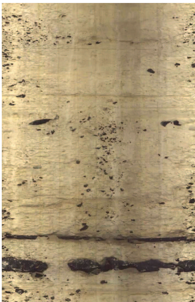
Oriented unwrapped optical televiewer image showing flint bands in chalk.
