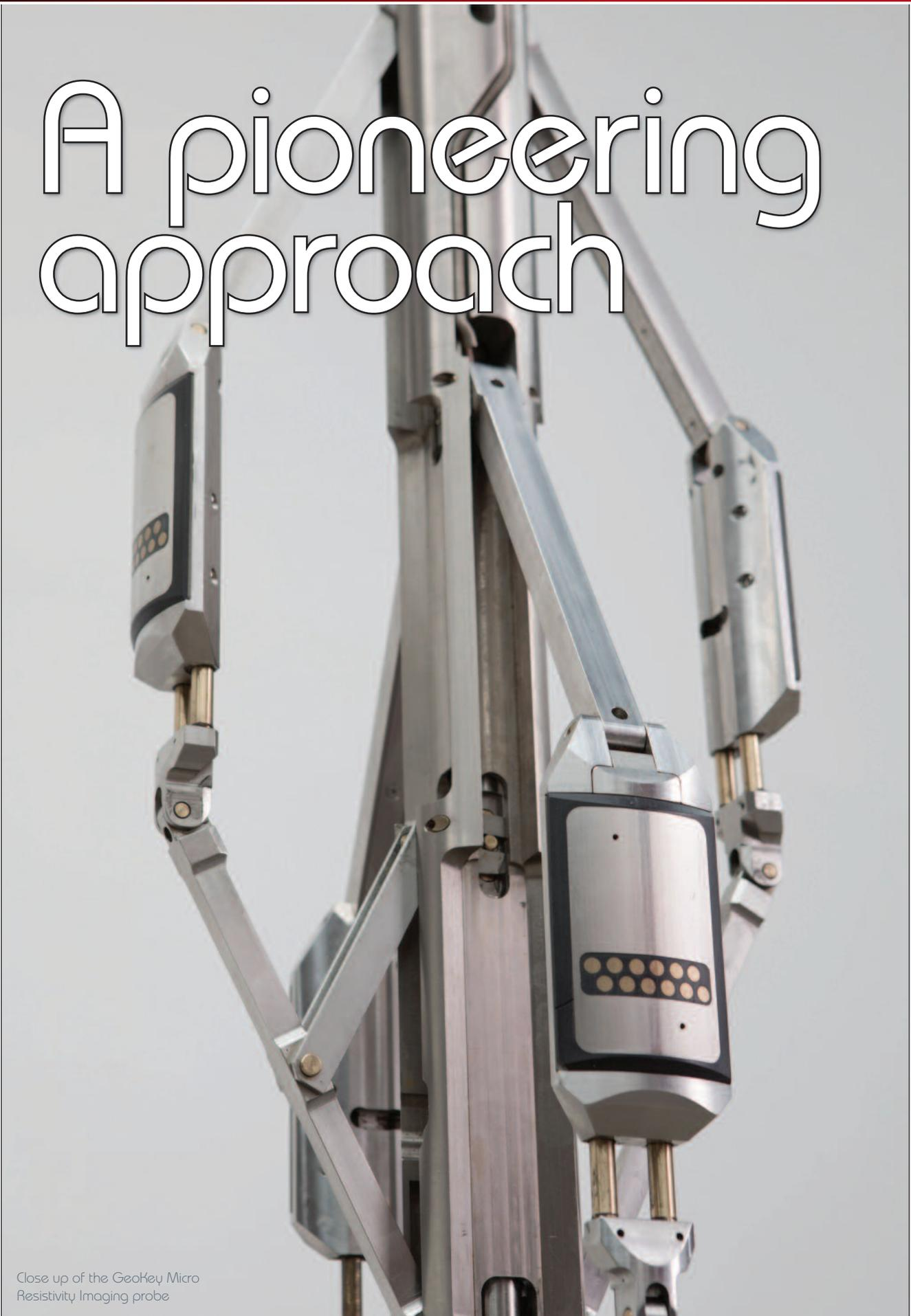
Close up of the GeoKey Micro Resistivity Imaging probe
