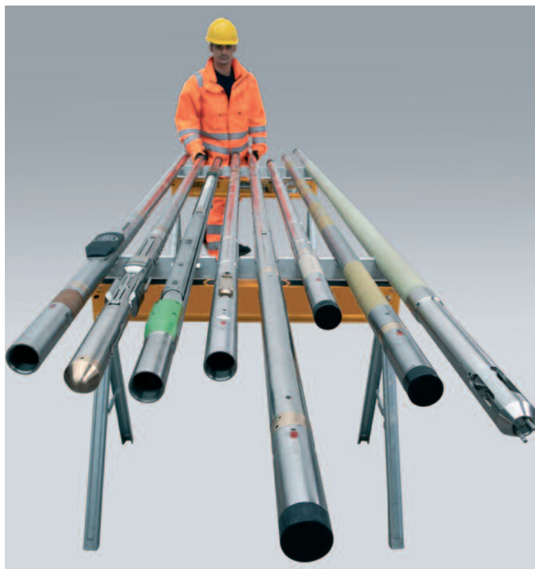
Figure 4. A complete GeoKey Logging system.
